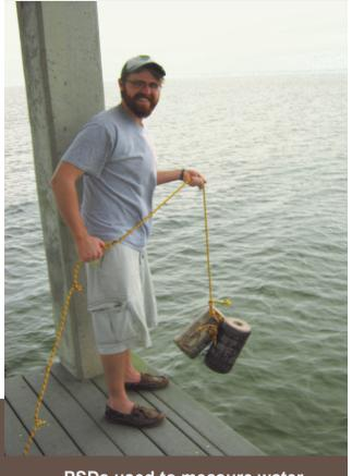
PSDs used to measure water quality are secured to a pier in cages and placed in the water.
