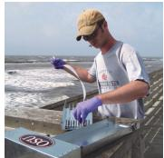
A researcher loads a PSD in a cage to measure the air quality.
